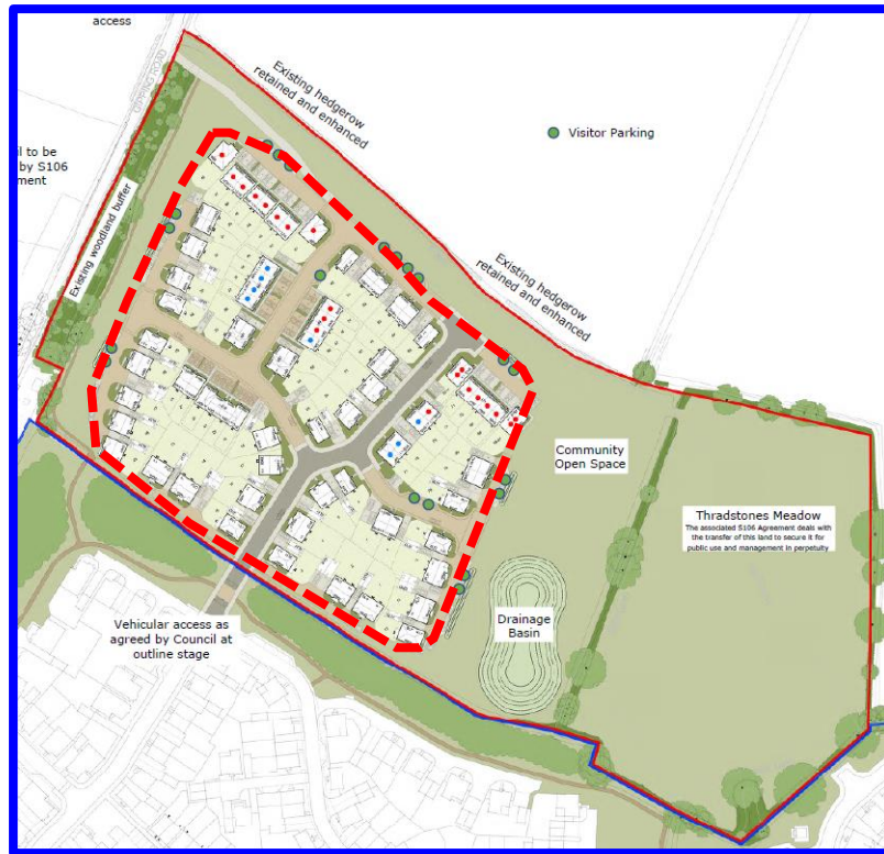
figure 8: Proposed layout with restricted built area from outline pp. shown in red dashed line
